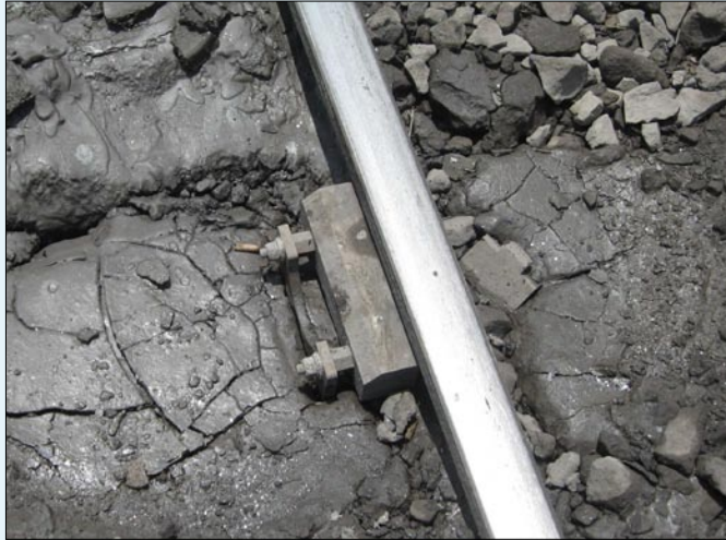
Figure 6: Wheel sensor under rough environmental conditions
