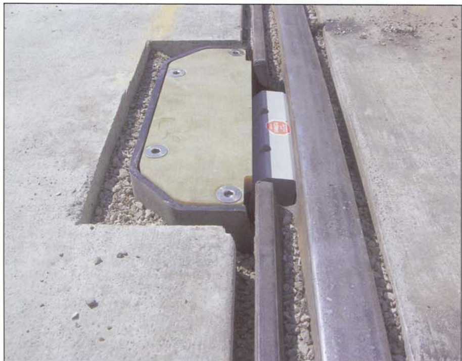
Figure 1: Wheel sensor RSR180 mounted to grooved rail claw (without rubber cap)
